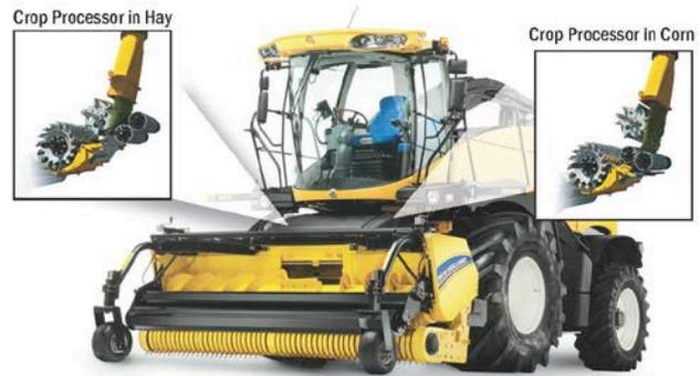
The Variflow™ system adjusts chopping to crop conditions: virtually eliminating plugging and saving horsepower.
