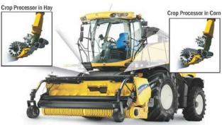
The Variflow<sup>™</sup> system adjusts chopping to crop conditions: virtually eliminating plugging and saving horsepower.
