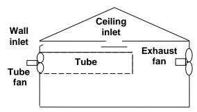
Figure 1. Schematic of a mechanically ventilated barn with a tube system
